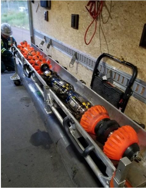
ILI tools, courtesy of Xcel Energy.
