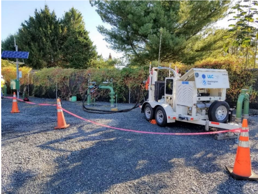
Temporary Draw Down Compressor for Medium Scale Projects, courtesy of Ryan N. Miller, Washington Gas.
