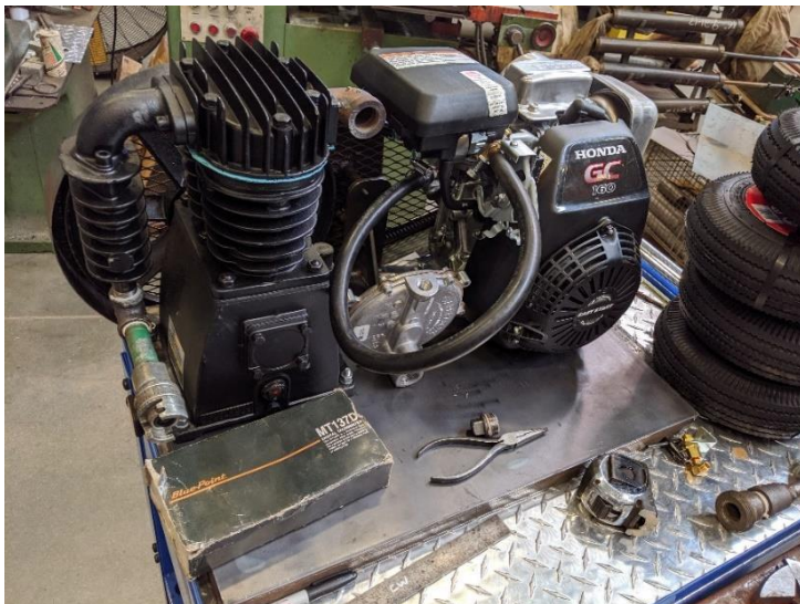
Prototype Temporary Draw-Down Compressor for Small Scale Projects (Small Mains and Services), courtesy of Ryan N. Miller, Washington Gas.
