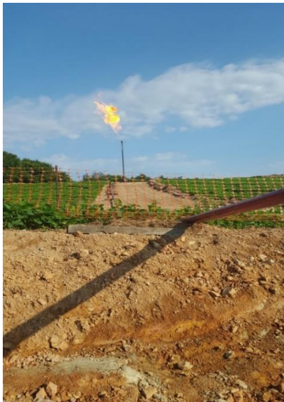
Blowdown Flares in operation, courtesy of Barry Smith, General Manager, Farr Front Chemical Services.
